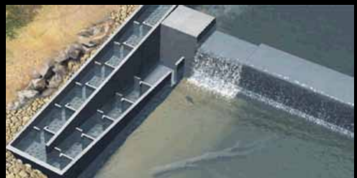
Conceptual illustration of vertical slot fishway at a weir showing chambers of the 'ladder' structure that enables fish to move up the river.
